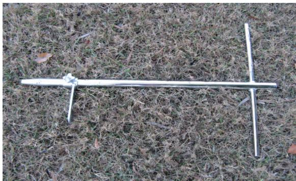
***A deep sample 'auger' type sampling probe.***
