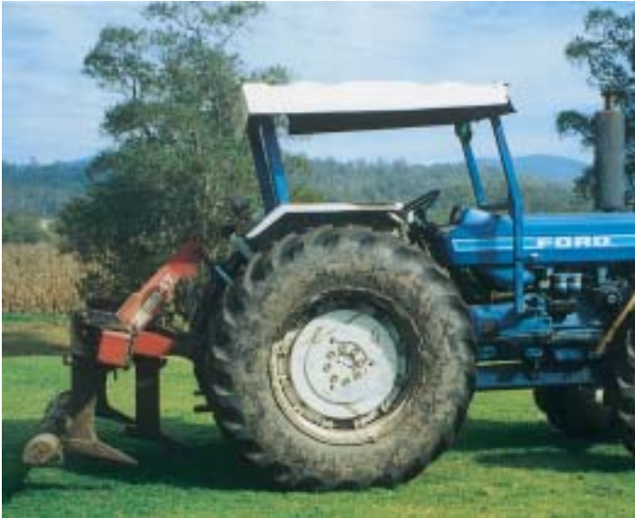
A deep ripper for shattering a 'hardpan' layer.
