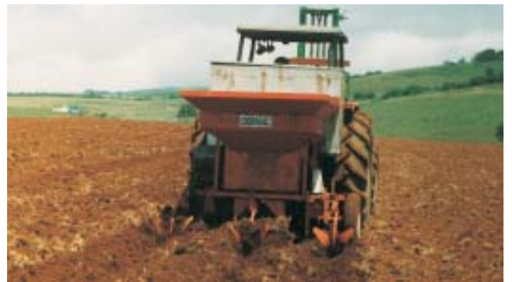
Machines that hill and plant in the one operation help reduce the number of soil workings.
