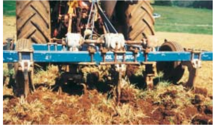
One pass with this 'Power Harrow' over sprayed-off pastures can produce a suitable seedbed for potatoes 1 .
