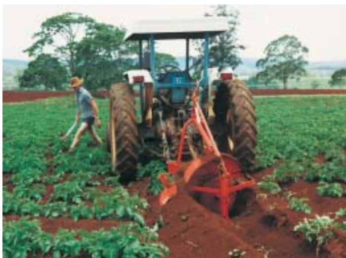
A rotary drain digger making temporary erosion control banks in a potato crop.
