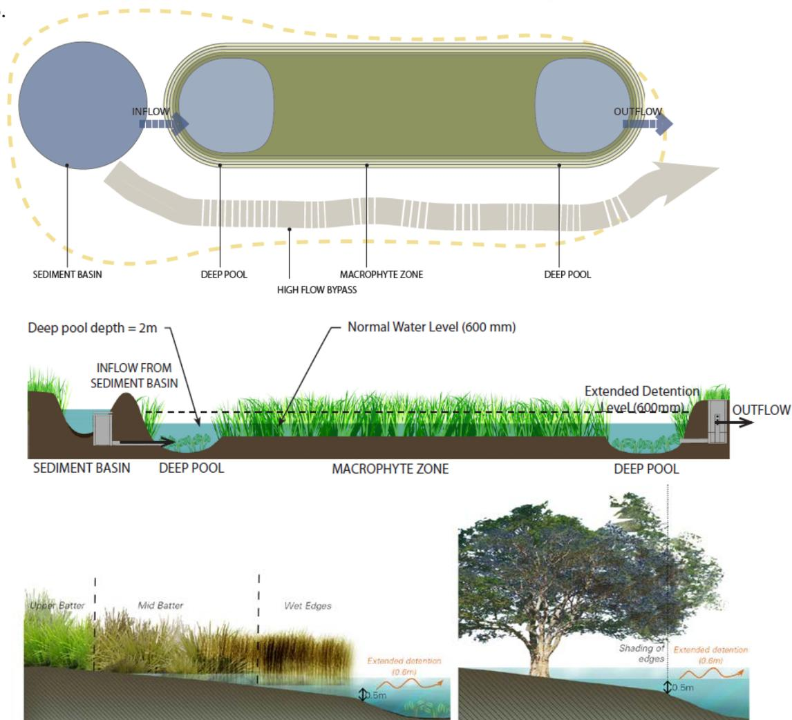
Figure 2 - Wetland plan view (top) and cross section (middle) and potential edge treatments for weed management (bottom).
