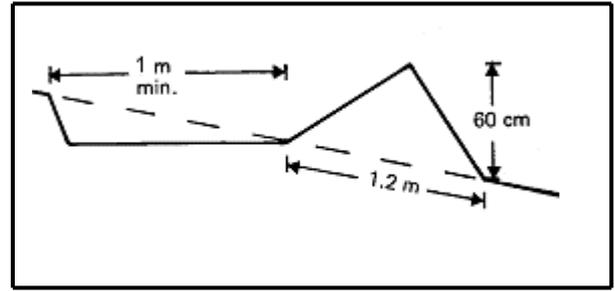
Figure 2: Cross-section of flat-channelled bank
