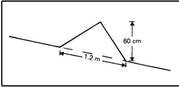
Figure 1: Cross-section of a contour bank
