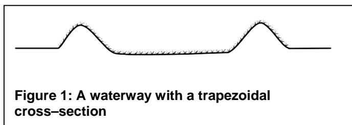
**Figure 1: A waterway with a trapezoidal cross-section**
