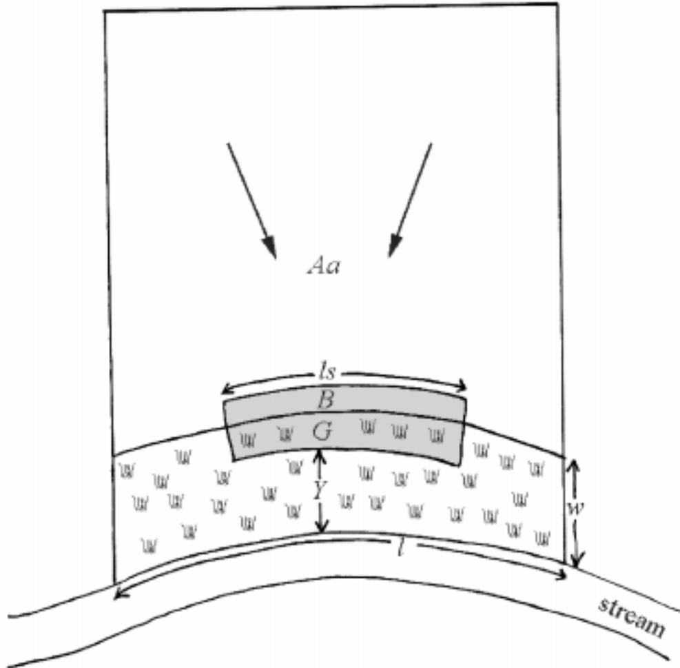
Figure 5. Definition of riparian filter strip at the bottom of a paddock of area  $a$ , with annual soil loss  $A$ .  $B$  = backwater sediment mass;  $G$  = grass sediment mass;  $w$  = filter width;  $l$  = filter length;  $l_s$  = length of deposit and  $Y$  = additional width required for settling sediment.
