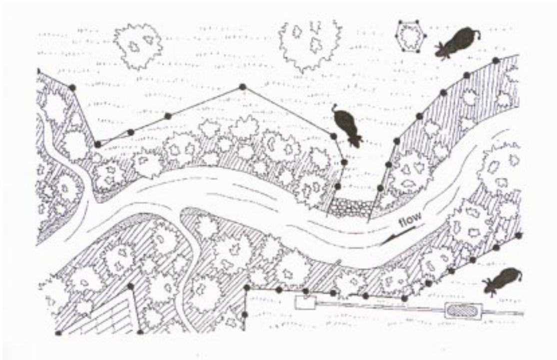
Figure 6. Two types of controlled stock access: a restricted access point (top of diagram) and an off-stream watering point (bottom of diagram). (DNR, 1998).
