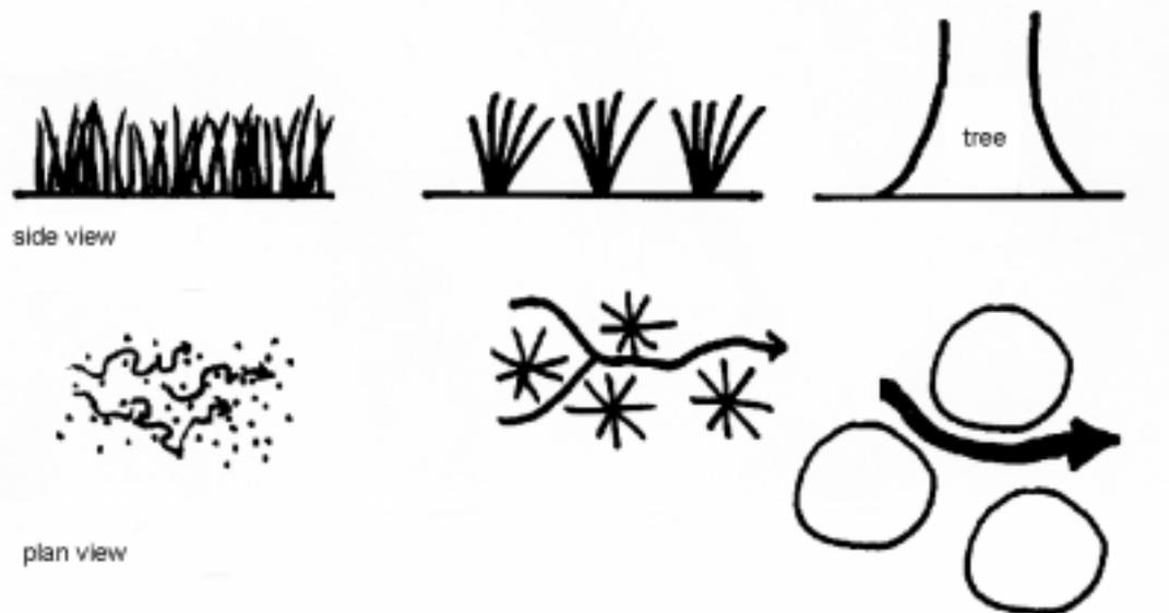
Figure 2. The vegetation density at ground level, and the way it can diffuse and slow down the flow are the main properties for filter strip vegetation. Dense, stoloniferous grass has the best properties for sediment trapping. (Thickness of arrow indicates flow velocity).
