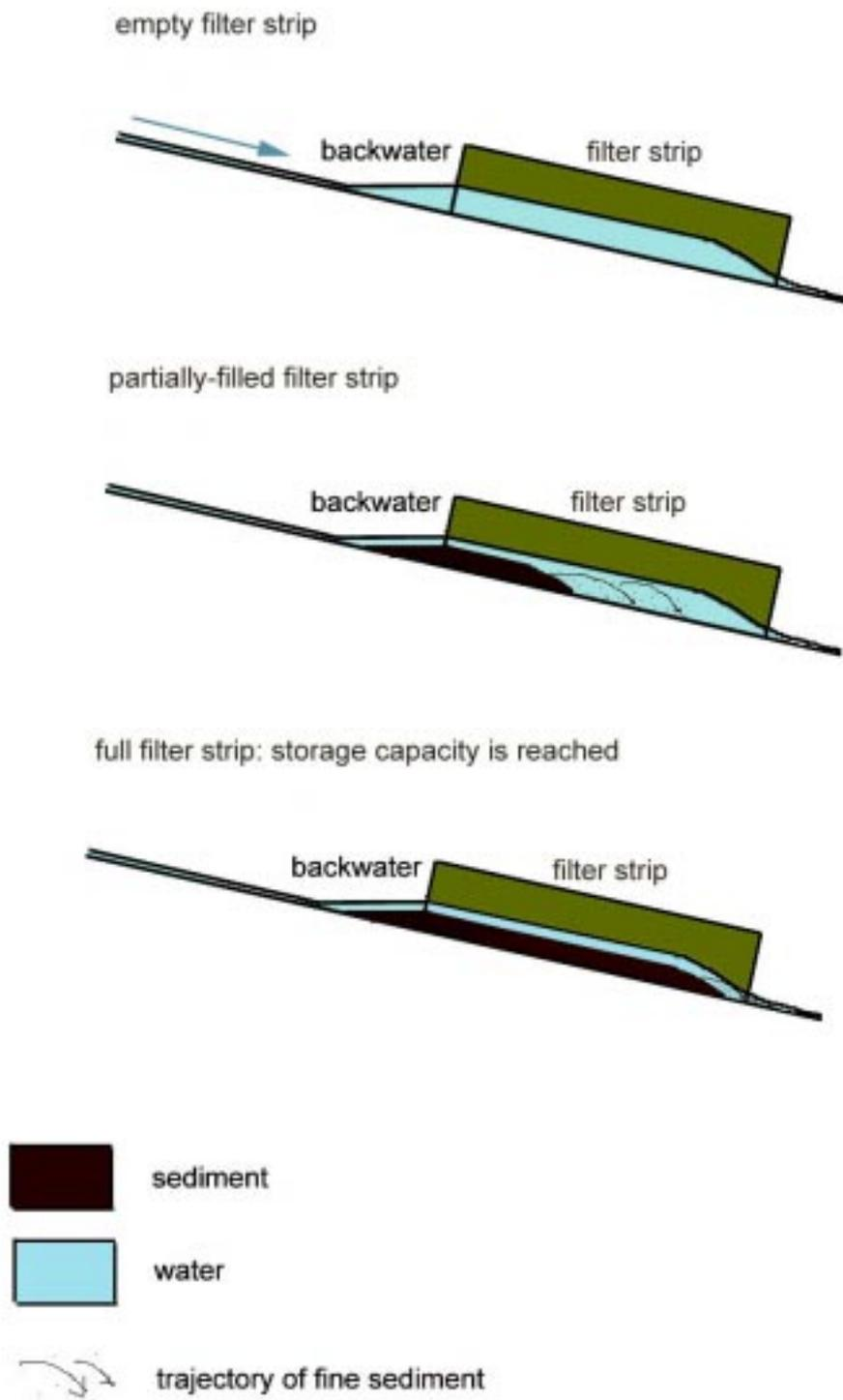
Figure 1. Grass filter showing backwater with forward growing deposit during trapping event.
