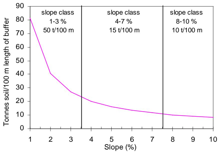
Figure 4. Backwater storage changes with slope of the grass filter. Based on unpublished experiments at CSIRO Land and Water, February 1999.
