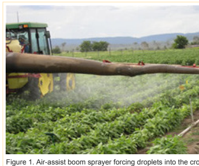
Figure 1. Air-assist boom sprayer forcing droplets into the crop
