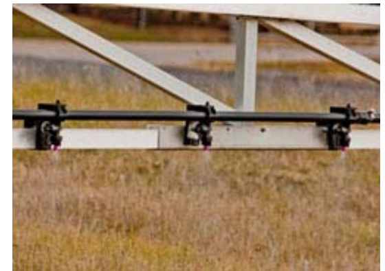
Boom fitted with purple nozzles
