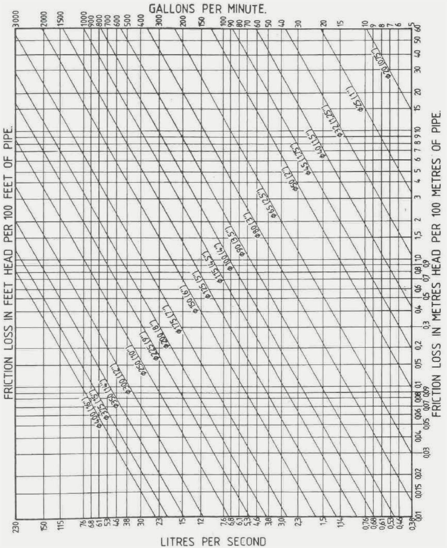
Figure 2: Discharge pipeline friction
