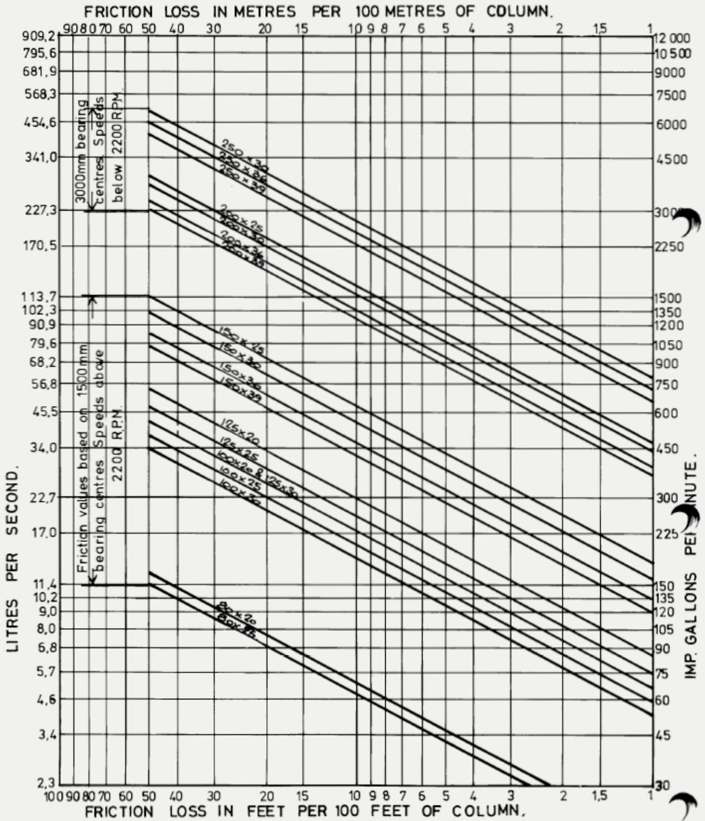
**Figure 3: Water Lubrication: Column Capacity Chart – Standard Col-Shaft Dimensions**
