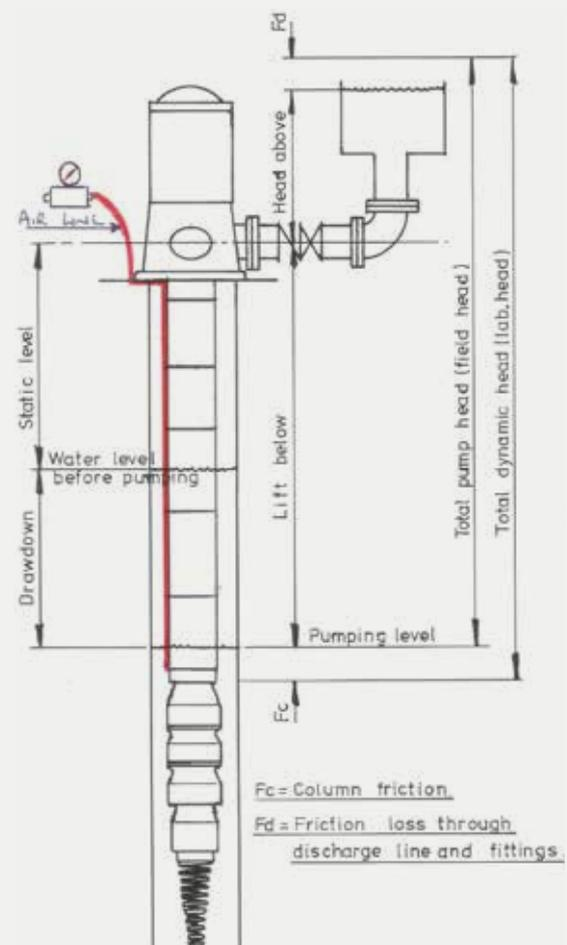
**Figure 1: Total Dynamic Head Diagram**
