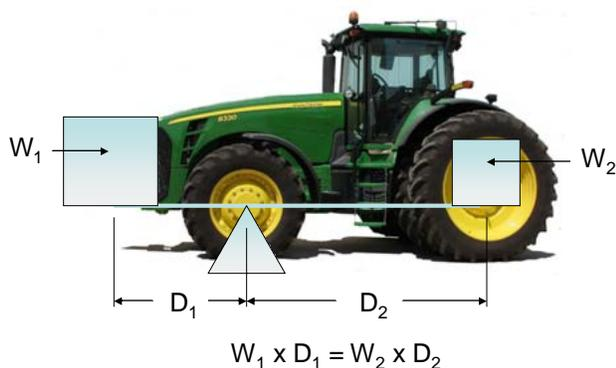
For example, how will the axle weights change if 600 lbs. in suitcase weights ( $W_1$ ) are added, the distance between the center of the suitcase weights and the center of the front axle is 6' ( $D_1$ ) and the distance between the front and rear axles is 10' ( $D_2$ )? Insert these values into the formula in figure 1.
