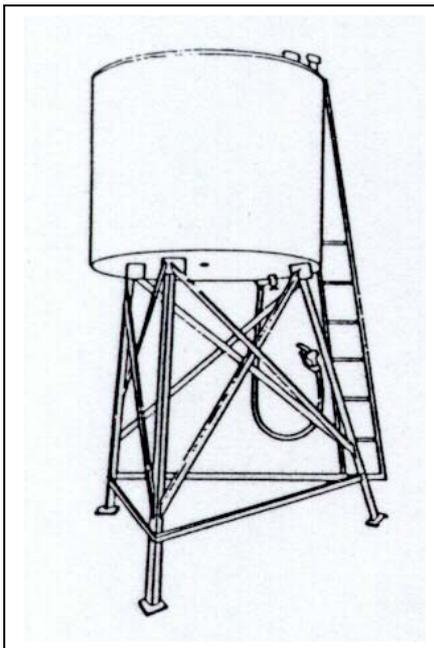
Tripod supporting structures are the least desirable for fuel storage tanks due to their inherent instability. Tripod stands are not to be used on tanks greater than 2200 litre capacity. Particular attention needs to be paid to tripod tank supports to ensure that they are in sound structural condition and that they have adequate footings (as above).
