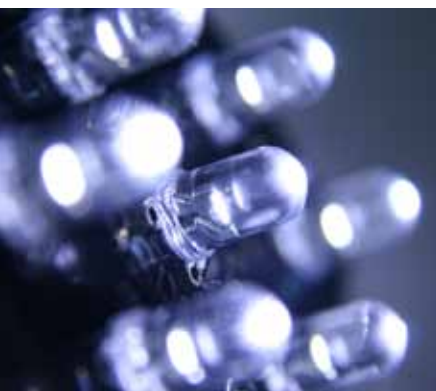
LEDs are very energy efficient as they convert electrical energy directly into a coloured light generating very little heat.
